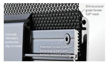
All Crimsafe products feature our patented Crimsafe Screw-Clamp™ technology. Tamper resistant screws first go through a metal clamp, then through Crimsafe's Tensile-Tuff® mesh and then driven right into the frame, to hold the mesh in a "vice like" grip. This patented Screw-Clamp® gives Crimsafe screens enormous strength against attack, unlike inferior products that simply glue or wedge mesh into a frame.
